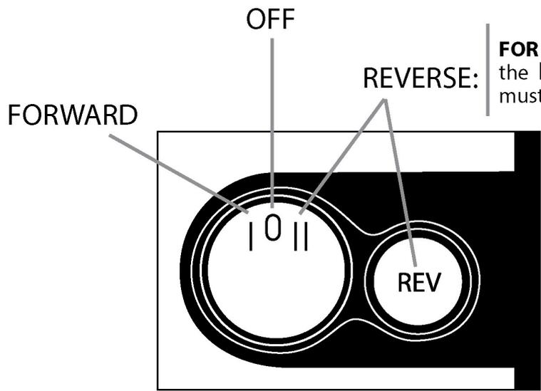
**FOR REVERSE:** Turn Knob to the II position. REV button must be pressed down also.
